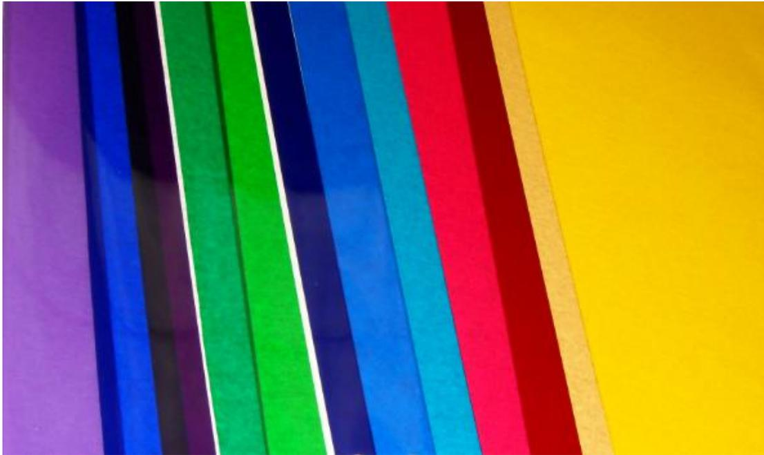
*Figure 3.11: Lighting gel filters used for polychromatic SR method*
