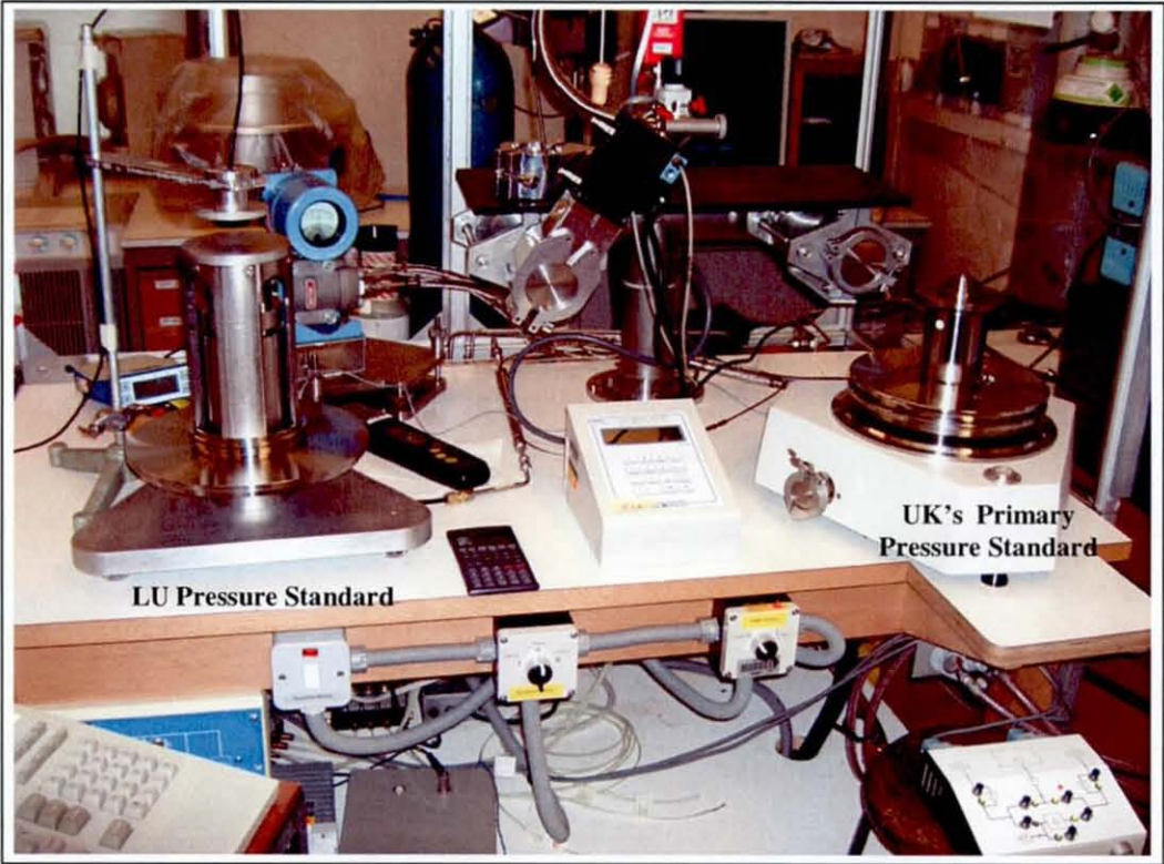
FIGURE 9.4 Cross floating experiment against the UK's Primary Pressure Standard
