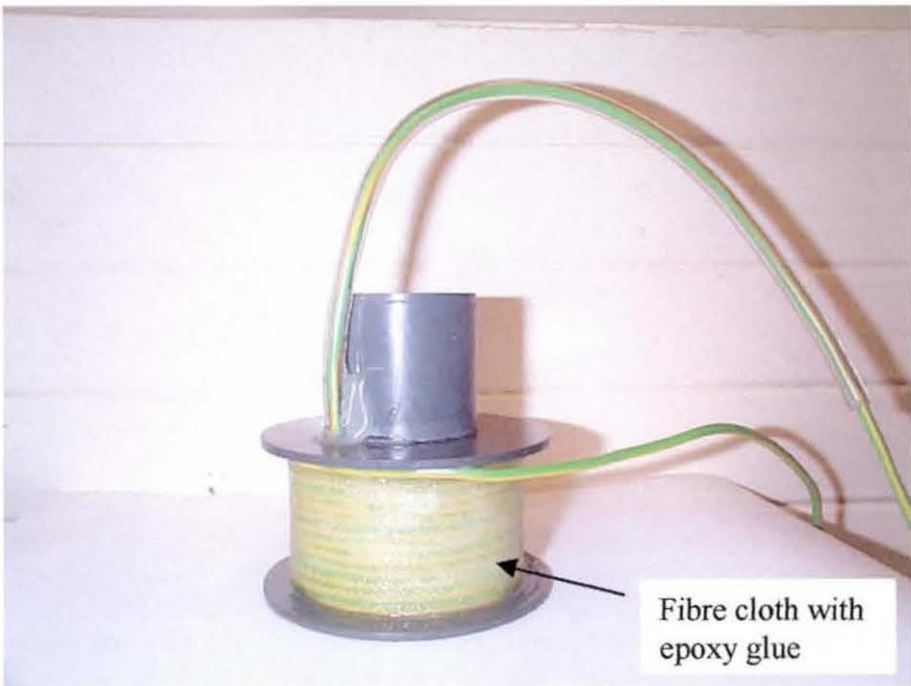
Figure B-3 Step – 3, Secure completed windings with fibre cloth and epoxy glue.
