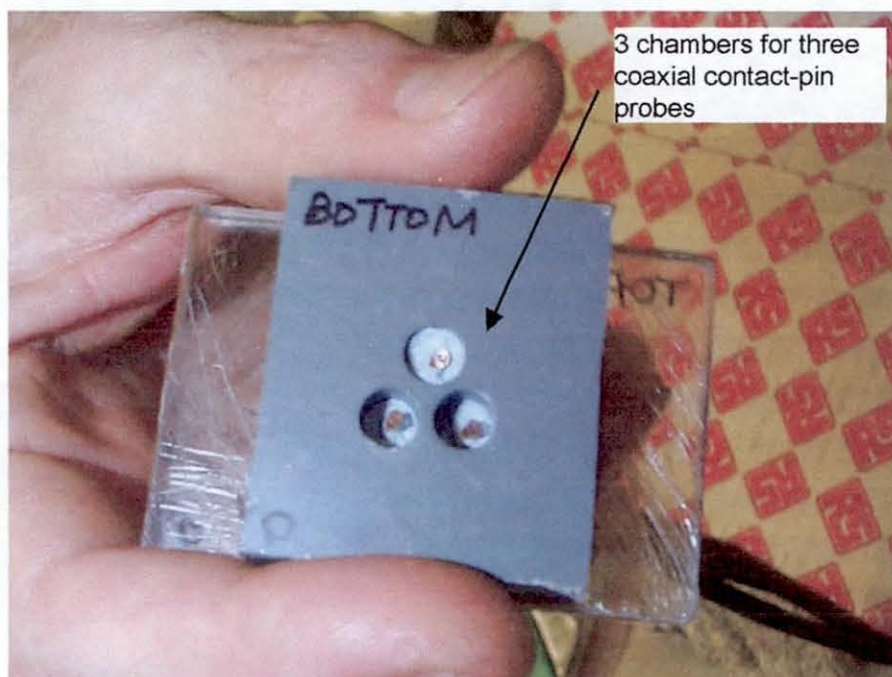
Figure 5-6 Coaxial contact-pin probes for multiple TOA measurements.
