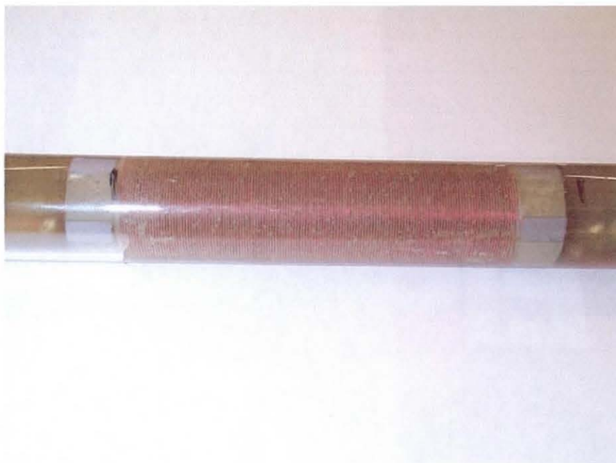
Figure 8-2 Epoxy-cast helical coil used for static transformer testing.
