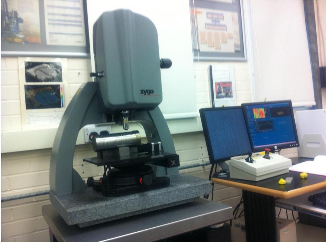
Figure 4-25: Experimental setup for surface roughness analysis using Zygo® interferometry
