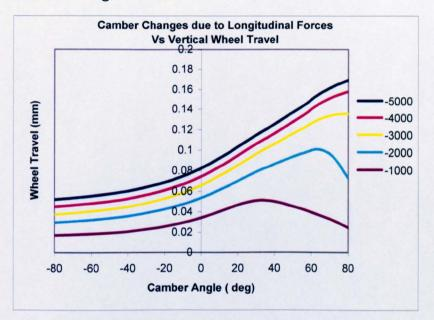
Figure 4.20a: Camber changes Vs vertical wheel travel due to longitudinal forces
