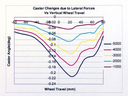
Figure 4.21b : Caster change Vs vertical wheel travel due to lateral forces
