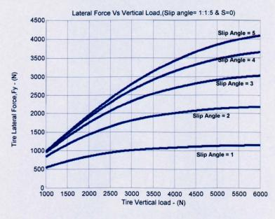
Figure 3.19: Lateral force Vs vertical load
