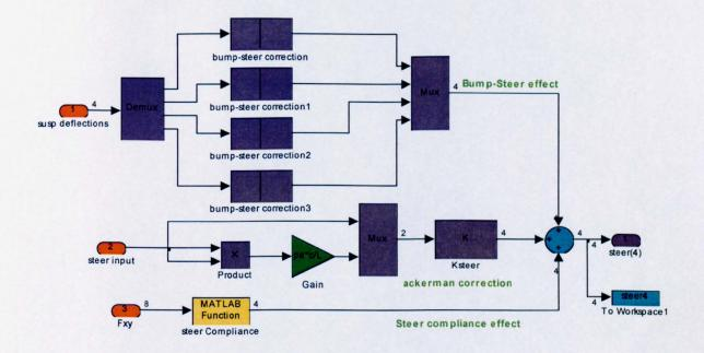
Figure 3.30 Suspension Motion Block
