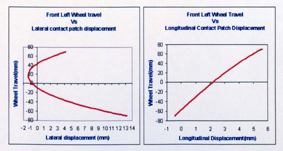
Figure 4.5: Wheel travel Vs Lateral/longitudinal displacement of at contact patch
