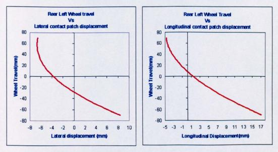
Figure 4.10: Vertical wheel travel Vs Lateral/longitudinal displacement at contact patch
