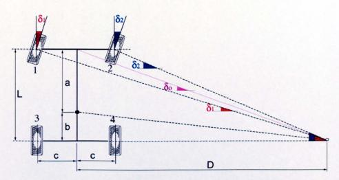
Figure 3.13: The Ackerman steering geometry
