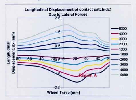
Figure 4.18b: Longitudinal deformation at contact patch due to Fy
