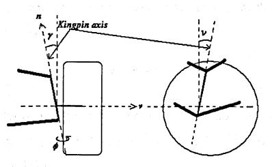
Figure 3.5: Virtual steering axis
