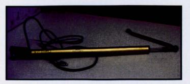
Figure 5.3: Vishay Precision Linear Transducer
