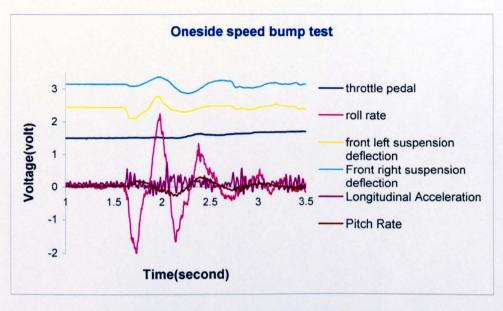
Figure 5.25: One side Speed Bump Test Result
