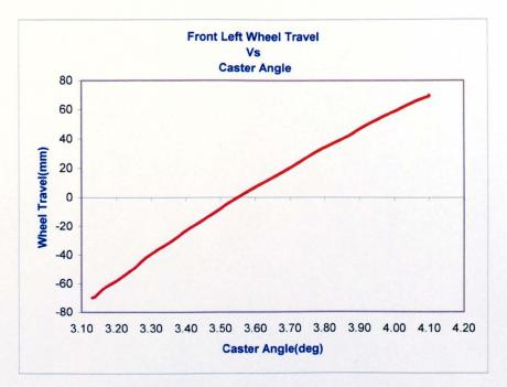
Figure 4.7: Vertical wheel travel Vs Caster Angle
