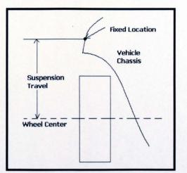
Figure 5.13: Measurement of suspension travel
