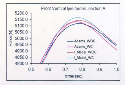
Figure 6.21: Section A - Front left vertical forces during transient condition
