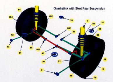
Figure 4.9: The Rear Suspension System
