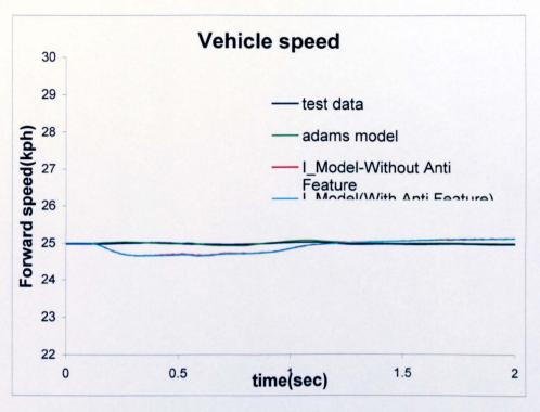
Figure 6.8b: Constant speedbump analysis, forward speed
