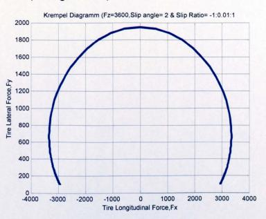
Figure 3.22: Lateral force Vs longitudinal force
