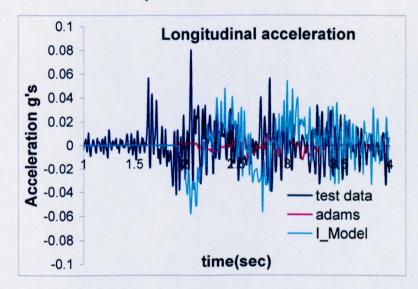
Figure 6.17a: Single speed bump analysis, longitudinal acceleration
