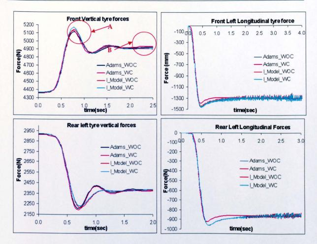
Figure 6.20: Front/Rear left vertical and longitudinal forces
