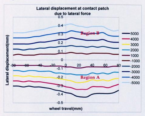
Figure 4.19b: Lateral deformation at contact patch due to Fy
