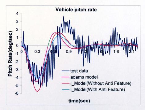
Figure 6.6a: Constant deceleration analysis, Vehicle pitch rate
