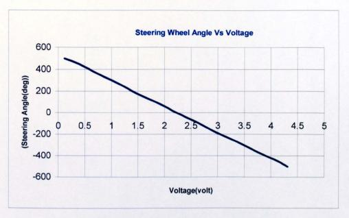
Figure 5.15: steering angle Vs voltage
