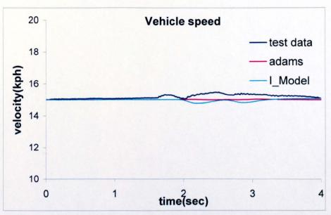
Figure 6.17b: Single speed bump analysis, forward speed
