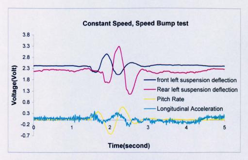
Figure 5.24: Speed Bump1 Test Results
