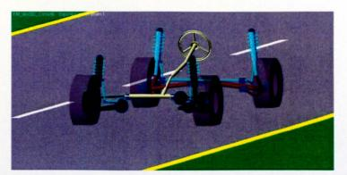
Figure 4.2: The ADAMS-base multi-body vehicle model
