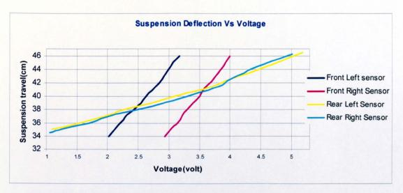
Figure 5.14: Suspension travel Vs voltage output (calibration curves)
