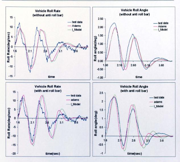
Figure 6.19: Variations in the roll rate and the roll angle
