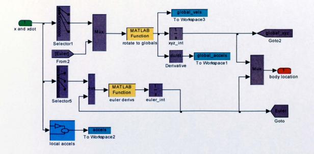
Figure 3.28 Vehicle kinematics block
