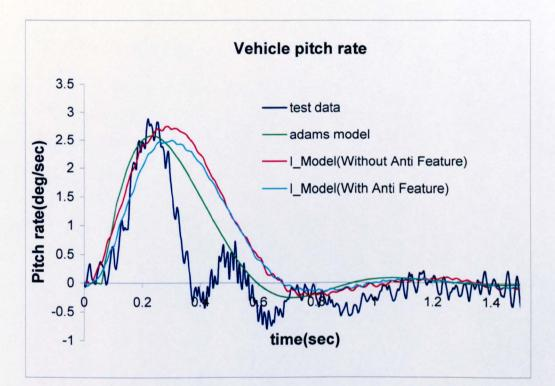
Figure 6.3a: Constant acceleration analysis, pitch rate
