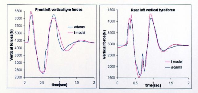
Figure 6.11: vertical tyre forces
