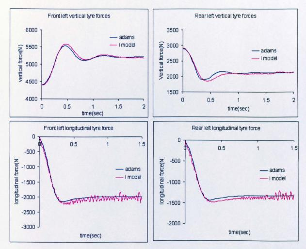
Figure 6.7: vertical and longitudinal tyre forces
