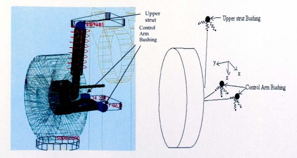
Figure 3.6: The McPherson Suspension system
