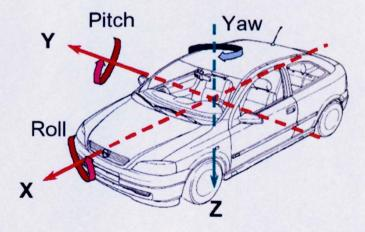
Figure 3.1: SAE Vehicle Axis Systems
