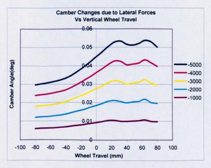
Figure 4.20b: Camber changes Vs vertical wheel travel due to lateral forces
