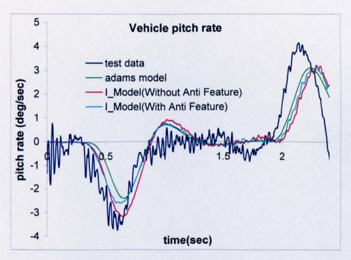
Figure 6.15a: Brake bump analysis, vehicle pitch rate
