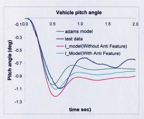
Figure 6.6b: Constant deceleration analysis, Vehicle pitch angle
