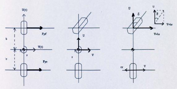
Figure 1.1: Free body diagram of the bicycle model
