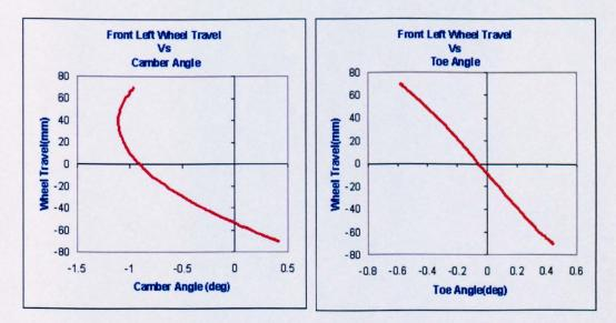
Figure 4.6: Vertical wheel travel Vs Camber/toe Angle
