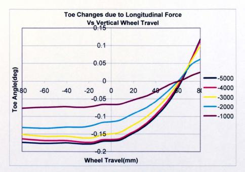
Figure 4.22a: Toe change Vs vertical wheel travel due to longitudinal forces
