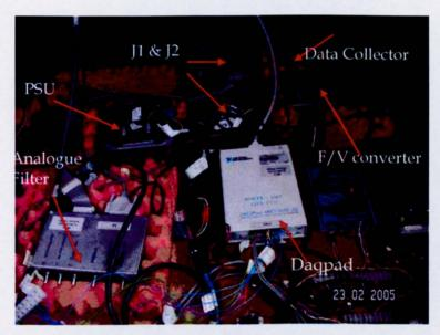
Figure 5.18: Data acquisition system located in the vehicle boot
