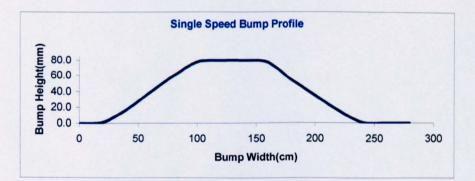
Figure 5.22: The single speed bump profile
