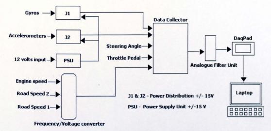
Figure 5.17: Schematic diagram of data logging system
