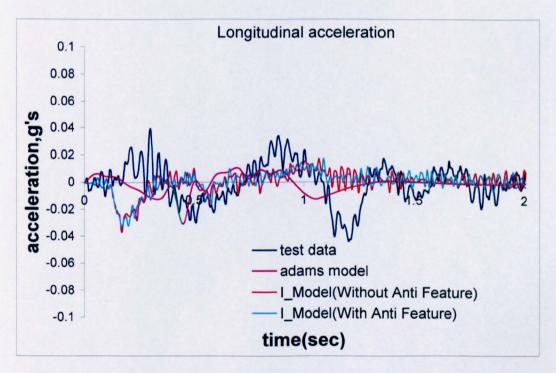
Figure 6.8a: Constant speed bump analysis, longitudinal acceleration
