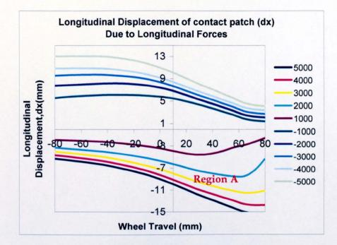
Figure 4.18a: Longitudinal deformation at contact patch due to Fx
