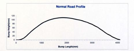
Figure 5.23: The normal speed bump profile
