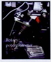
Figure 5.8: Potentiometer for measuring the steering angle
