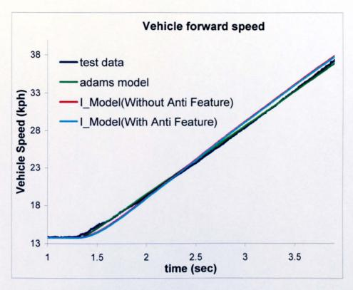
Figure 6.1b: Constant acceleration analysis, forward speed
