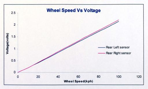
Figure 5.16: Wheel speed Vs voltage
