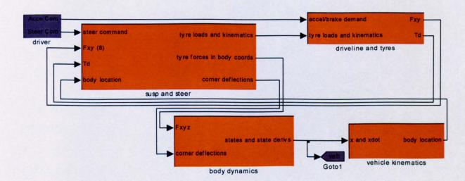
Figure 3.26 Overall vehicle dynamics model in MATLAB/SIMULINK environment
