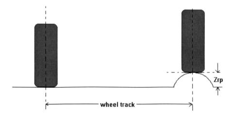
Figure 3.11: road profile effect on body roll
