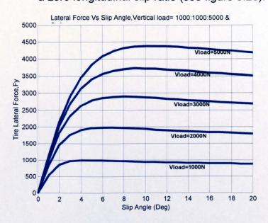
Figure 3.20: Lateral force Vs slip angle
