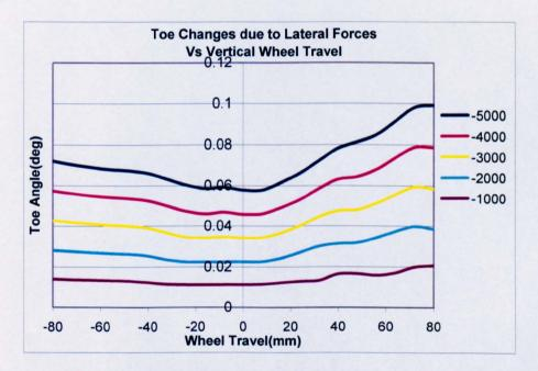
Figure 4.22b: Toe change Vs vertical wheel travel due to lateral forces
