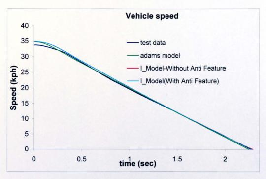
Figure 6.4b: Constant deceleration analysis , forward speed
