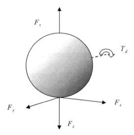
Figure 3.4: Forces and moments for the calculation of virtual work
