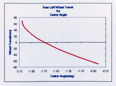
Figure 4.12: Vertical wheel travel Vs Caster Angle
