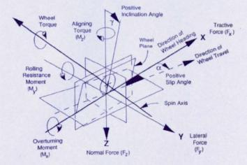
Figure 3.18: Tyre axes system(ADAMS/Pre, 2002)
