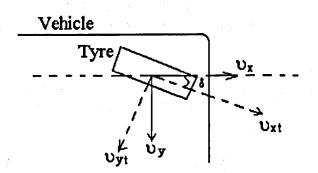
Figure 3.12: Velocity relative to the plane of vehicle
