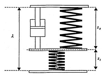
Figure 3.3: Tyre and suspension travel
