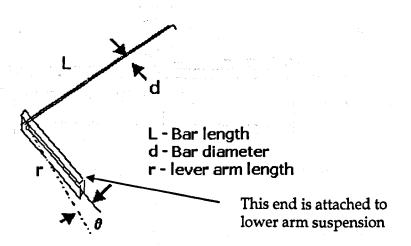
Figure 3.8: Twisting of the anti-roll bar
