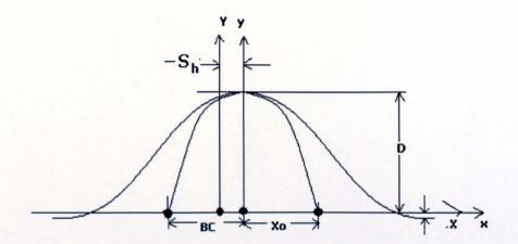
Figure 4.15: Some parameters in the tyre model (II)(ADAMS/Pre, 2002)
