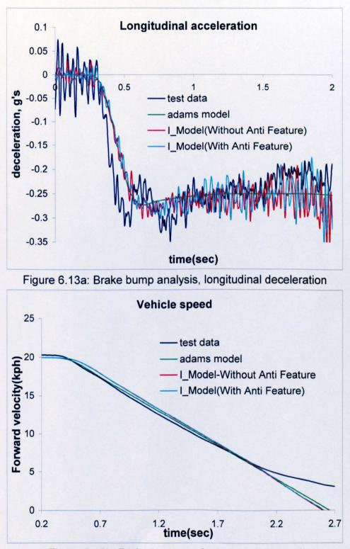
Figure 6.13b: Brake bump analysis, forward speed
