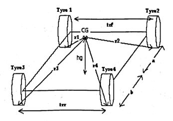
Figure 3.2: Notation used for each corner showing the distance from CG
