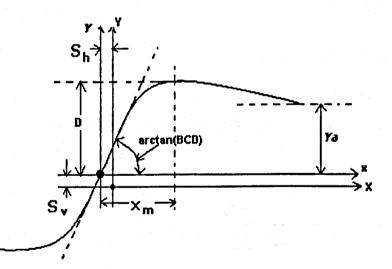
Figure 4.14: Some parameters in the tyre model (I)(ADAMS/Pre, 2002)
