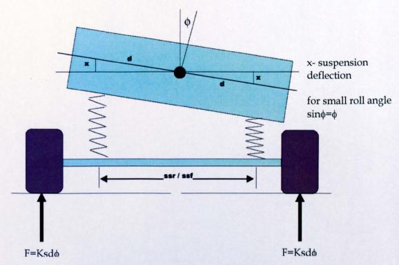
Figure 2.2: Suspension system for the 3-DOF model
