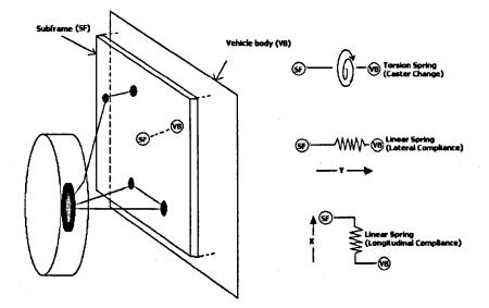
Figure 3.7: The simplified suspension compliance model
