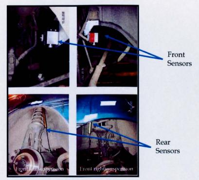
Figure 5.12: Installed front suspension displacement sensors
