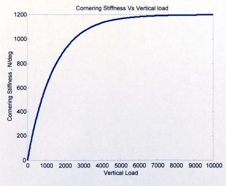
Figure 3.24: cornering stiffness Vs vertical load
