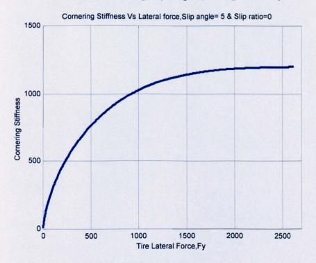
Figure 3.25: Cornering stiffness Vs Lateral force
