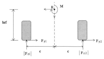
Figure 3.2: Vertical load
