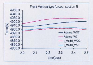
Figure 6.22: Section B - Front left vertical force during steady state condition
