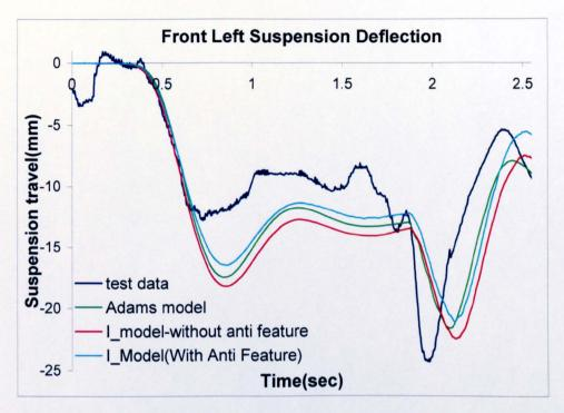
Figure 6.14a: Brake bump analysis, front left suspension deflection
