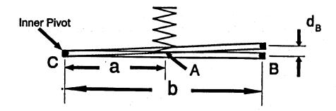
Figure 3.9: Suspension motion ratio
