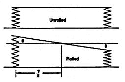
Figure 3.10: Vehicle body roll
