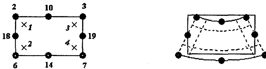
Figure 3.7 – Second Order Brick Element Definition and the Resolved Bending Problem.
