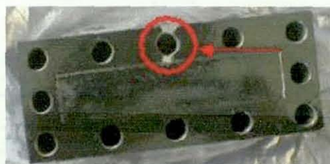
Figure 4.15 Gasket sealing failure.
