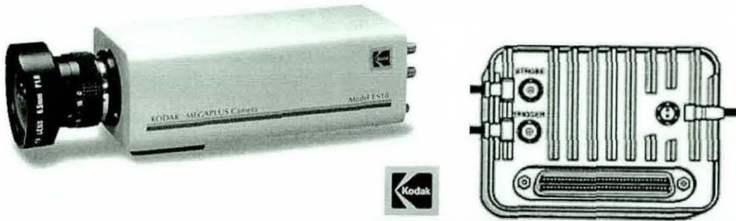
Figure 3.6 An image of the Kodak Megaplug camera with a C-mount lens.
