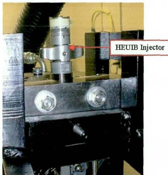
Figure 4.9 HEUIB injector mounted on the diesel optical rig.
