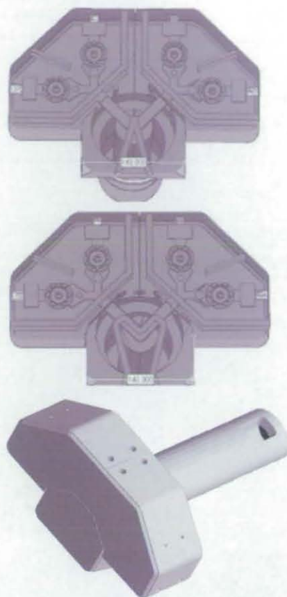
Figure 5 3D CAD models of the inserts and shot sleeve used for simulation
