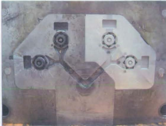
Figure 2 - MetalCopy & steel inserts in die-casting tool
