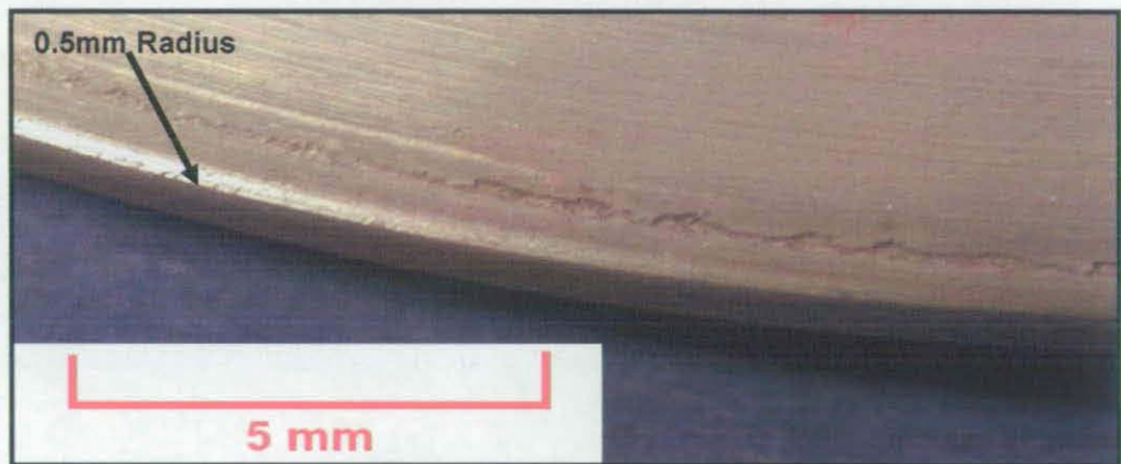
Figure 7 - 21 Horizontal laminate machining defects
