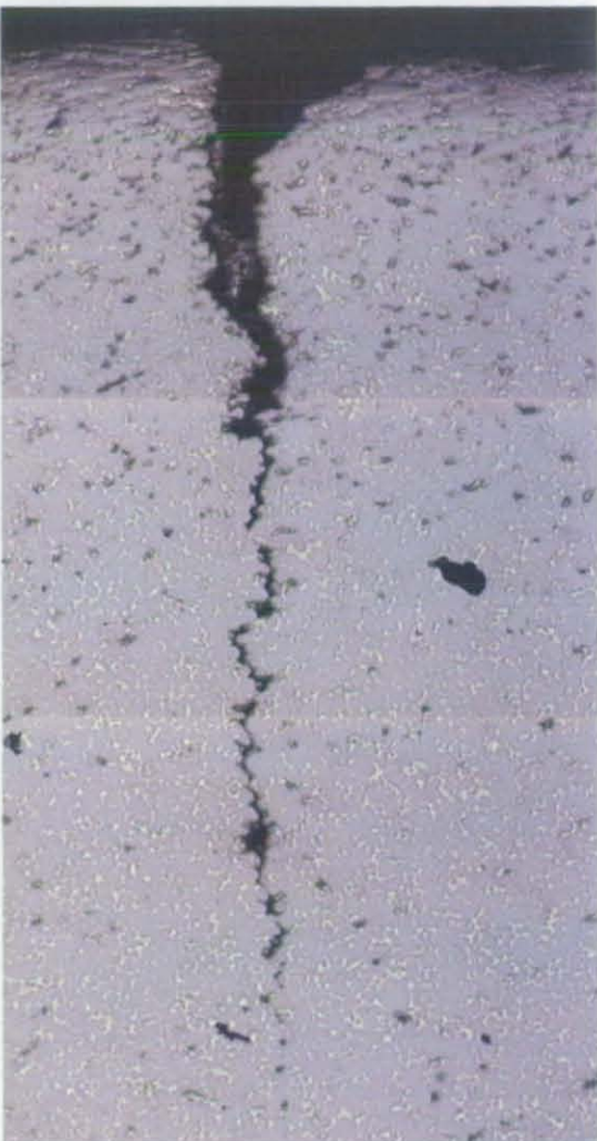
Figure 7 MetalCopy crack post casting
