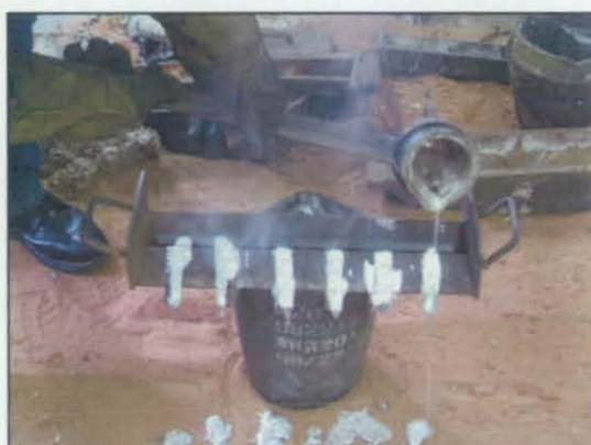
Appendix ii Figure 4 Aluminium being cast on the specimens
