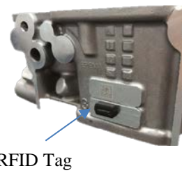
Figure 2. Cylinder Head with attached RFID tag
