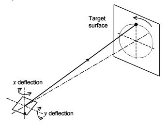
Figure 3 – The "ideal" scanning arrangement
