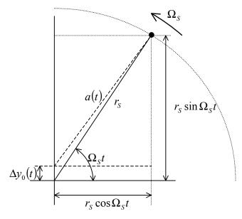
Figure 6 – Circular scanning profile projected onto a target
