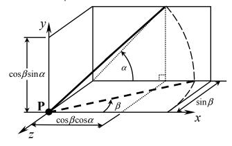
Figure 2 – Laser beam orientation, defining angles  $\alpha$  and  $\beta$
