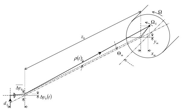
Figure 5 – Laser beam orientation for circular scanning profiles
