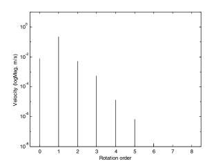
Figure 8 – Simulated frequency spectrum due to translational and angular misalignment in a circular tracking LDV system
