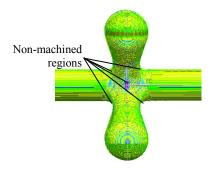
Fig. 1 Limited tool accessibility on part [9]
