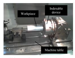
Fig. 5 Machining setups for CNC rapid manufacturing processes
