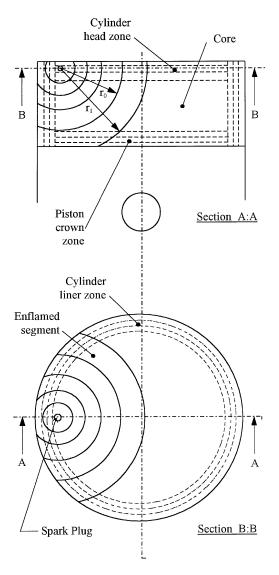
Fig. 1 Mass elements in a typical cylinder
