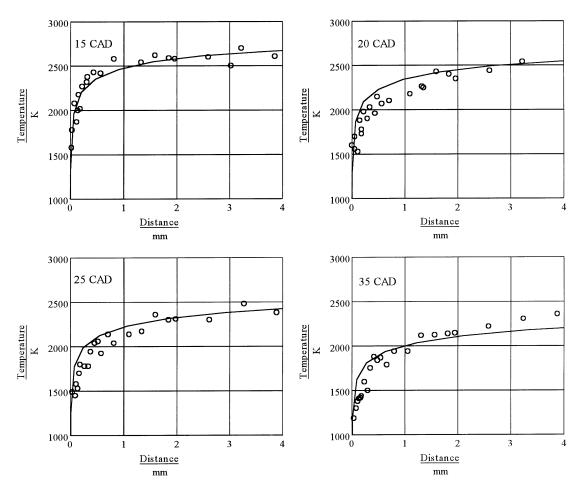
Fig. 8 Measured [11] and predicted burned gas near-wall temperature profiles at four crank angle positions
