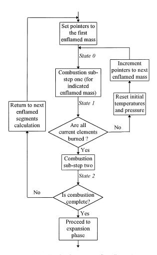
Fig. 2 Combustion process (flow diagram)
