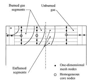
Fig. 3 Superimposition of one-dimensional grids and mass elements
