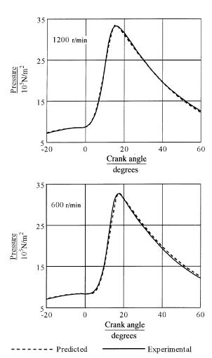
Fig. 6 Predicted and measured [13] pressure-crank angle diagrams for two engine speeds
