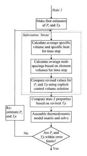
Fig. 4 Combustion substep 2 with heat transfer
