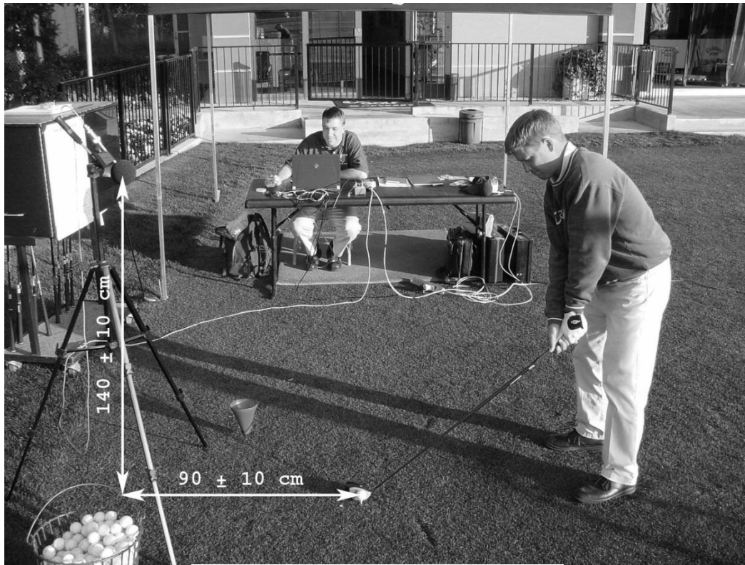
Figure 1. Microphone location in the test set-up
