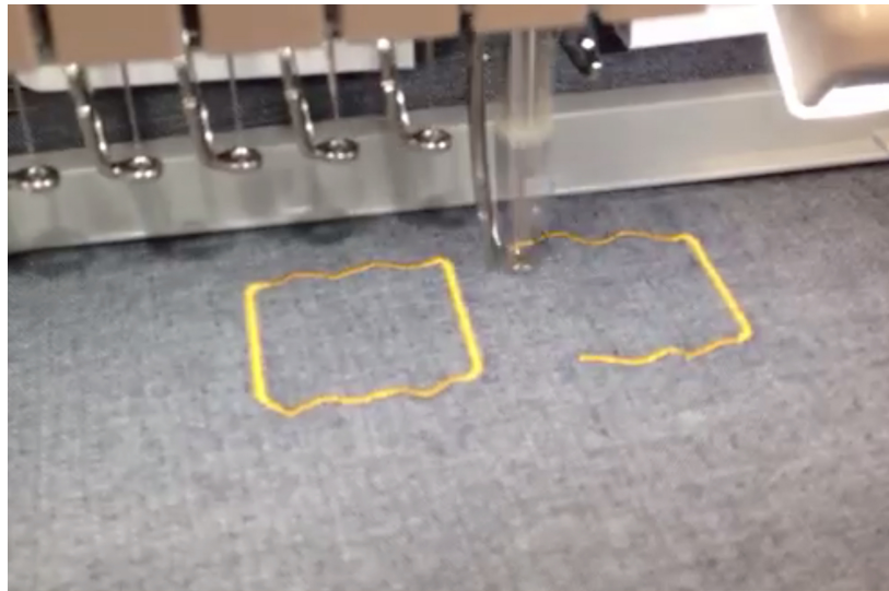
Figure 9. Embroidery machine creating FSS structure.
