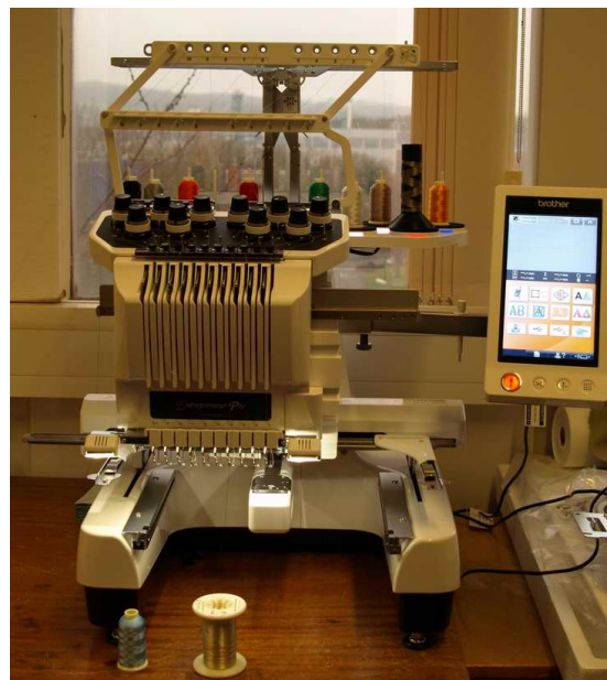
Figure 5. Computer aided embroidery machine at Loughborough University.
