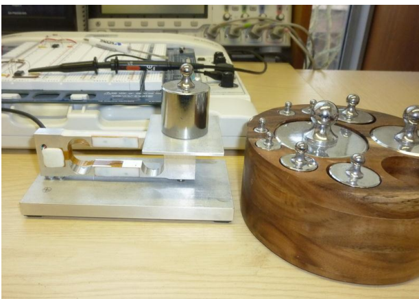
Figure 2. A load cell mounted and ready for use with the test weights
