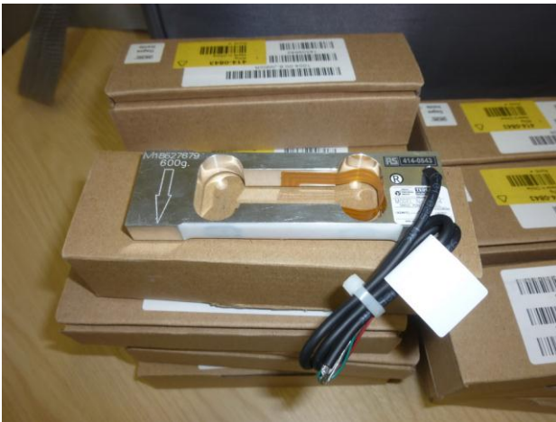
Figure 1. 25 load cells purchased for the project
