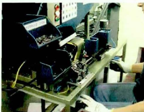
Figure 16. New assembly 05 station – Better design and double rate capacity.
