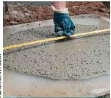
**Agilia™ Horizontal's finishing characteristics and high quality surface finish eliminate the need to power float concrete on site.**
