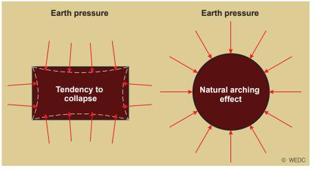
Figure 4. Stress concentrations on rectangular and circular pits
