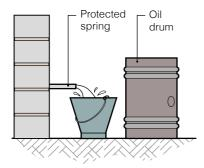
**Figure 34.** The types of containers communities use should inform the design of the water point
