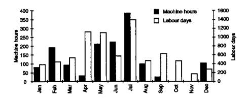
Figure 5.2 Canal Maintenance Inputs at Mwea Irrigation Settlement Scheme, 1992
