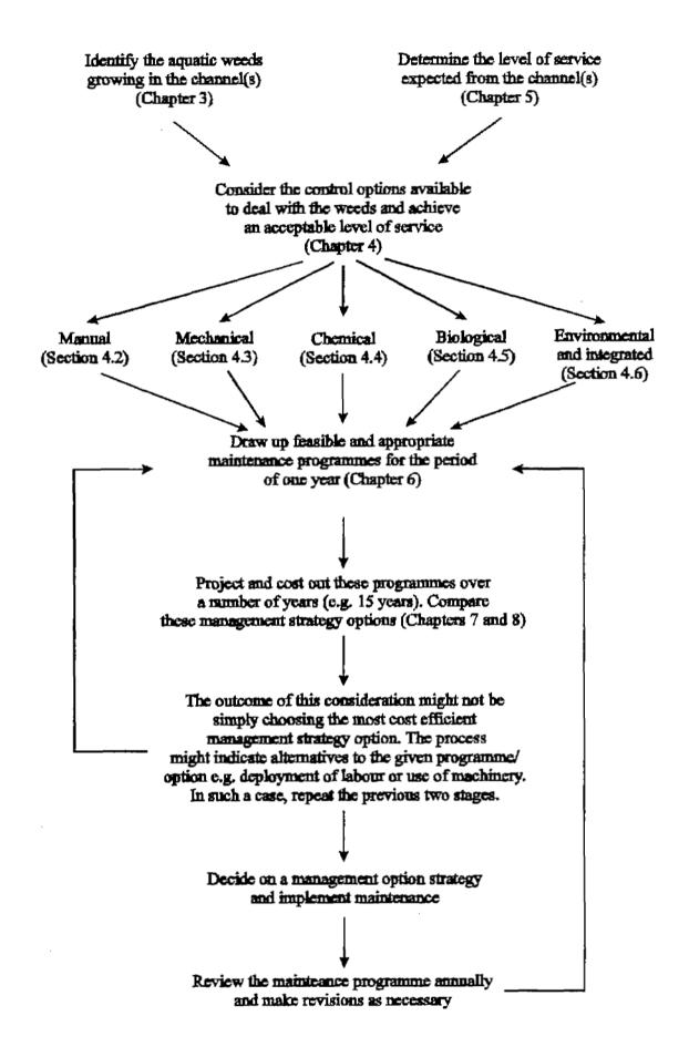
Figure 1.5. Process for determining aquatic weed maintenance strategy
