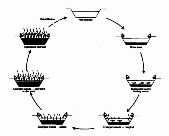
Figure 3.2. The stages of the hydroseral succession which occur in irrigation and drainage channels at Mwea Irrigation Settlement Scheme, Kenya
