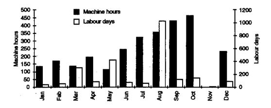
Figure 5.3 Drain Maintenance Inputs at Mwea Irrigation Settlement Scheme, 1992
