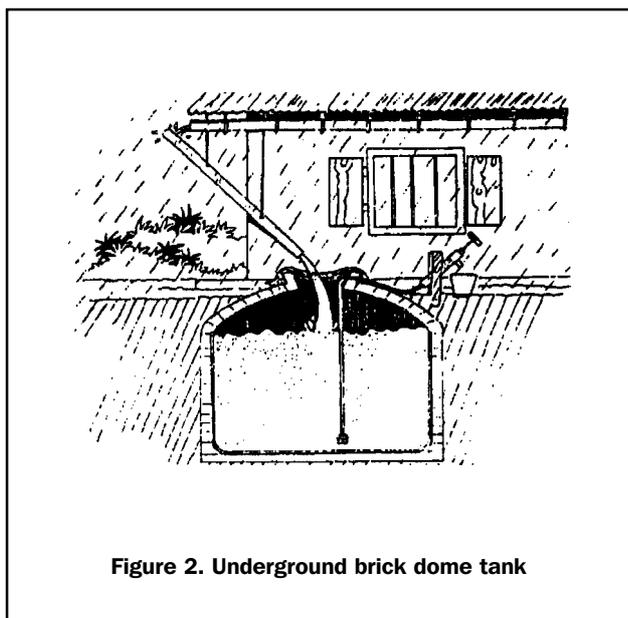
Figure 2. Underground brick dome tank
