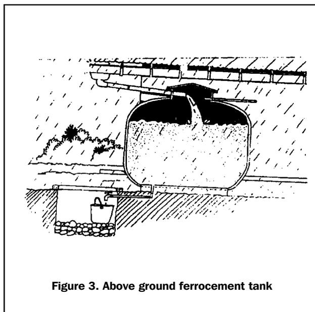
Figure 3. Above ground ferroceement tank
