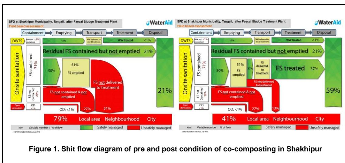
Figure 1. Shit flow diagram of pre and post condition of co-composting in Shakhipur
