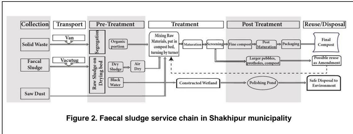
Figure 2. Faecal sludge service chain in Shakhipur municipality
