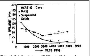
Figure 4. Relation between MLSS and efficiency of process
