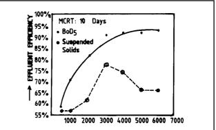
Figure 5. Relation between MLSS and efficiency process
