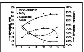
Figure 6. Relation between MCRT and efficiency of process
