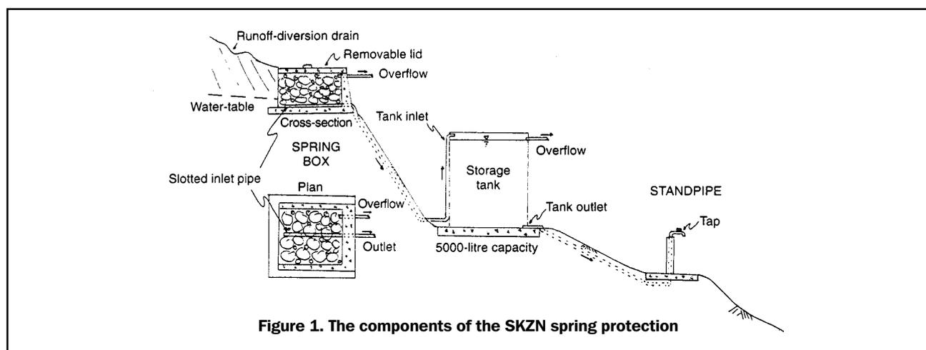
Figure 1. The components of the SKZN spring protection
