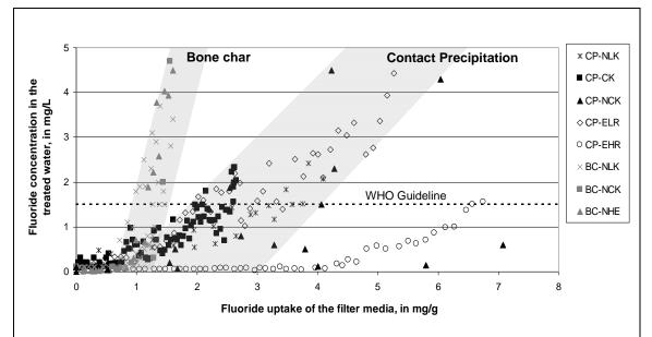
Figure 1. Fluoride uptake capacity of CP column experiments at CDN and Eawag, field tests on CP community filters maintained by CDN in Kenya (black symbols), and BC column experiments at CDN, field tests on BC community filters maintained by CDN in Kenya and BC household filters maintained by OSHO in Ethiopia (grey symbols)
