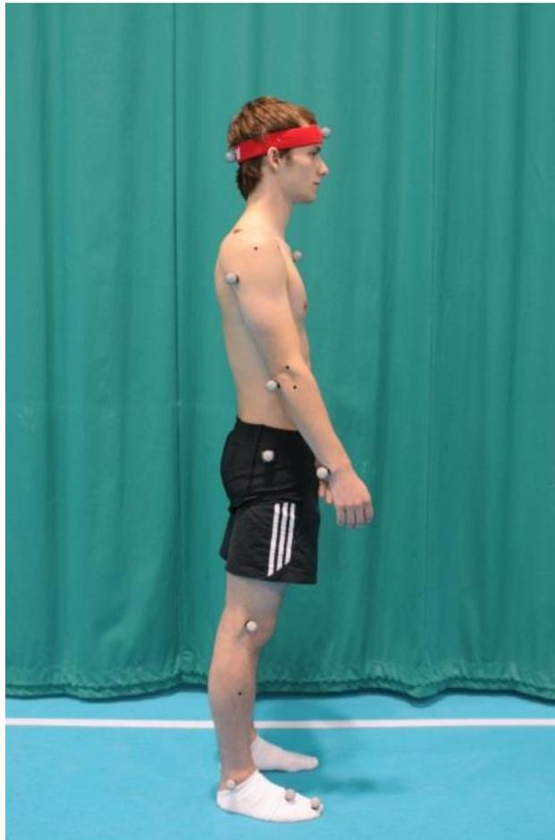
Figure 3.2.3 Photograph showing the marker set employed to collect position data.
