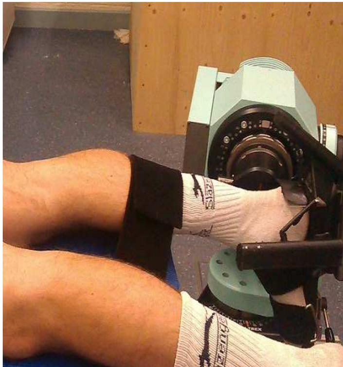
Figure 5.7: Dynamometer set up for ankle plantar flexion measurement
