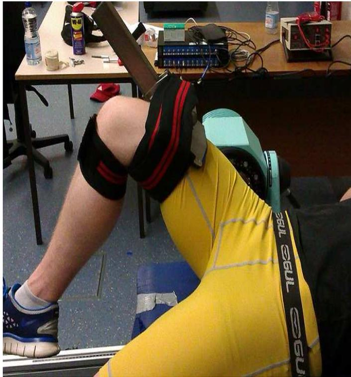
Figure 5.8: Dynamometer set up for hip flexion measurement
