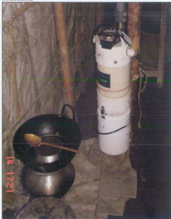
Figure 3.5: MiniVol and T28 machines placed near stove in a household
