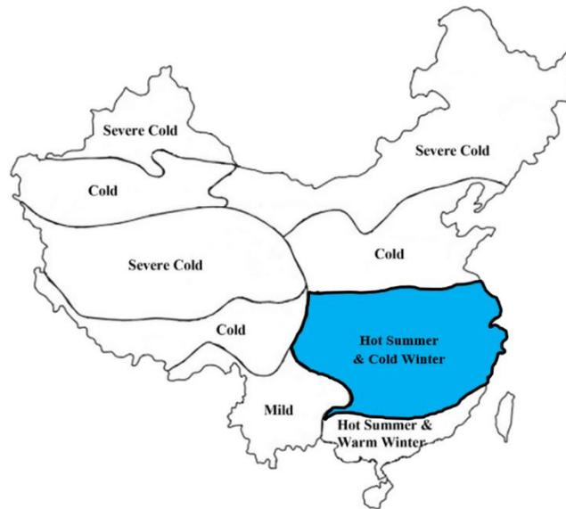
**Figure 1-1: Five climate zones for building design in China, with the studied Hot Summer and Cold Winter zone, highlighted in blue (adapted from Gou et al. 2015)**
