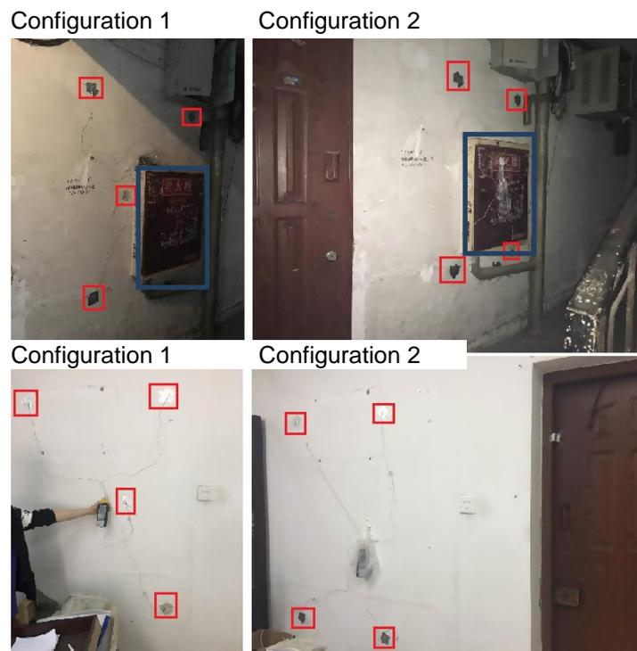
**Figure 4-11: Location of the thermocouples used to measure external wall temperature for two configurations, with red boxes showing thermocouples and blue boxes showing fire hydrant (source: Yao, 2017).**
